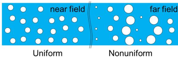
Fig. 2 Conceptual diagram of the result in Sec. 3.1: near field is initially monodisperse and far field is initially polydisperse.
