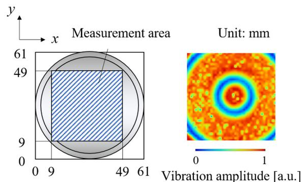
Fig. 2 Vibration amplitude distribution of the hemispherical vibration plate at 27.5 kHz.
