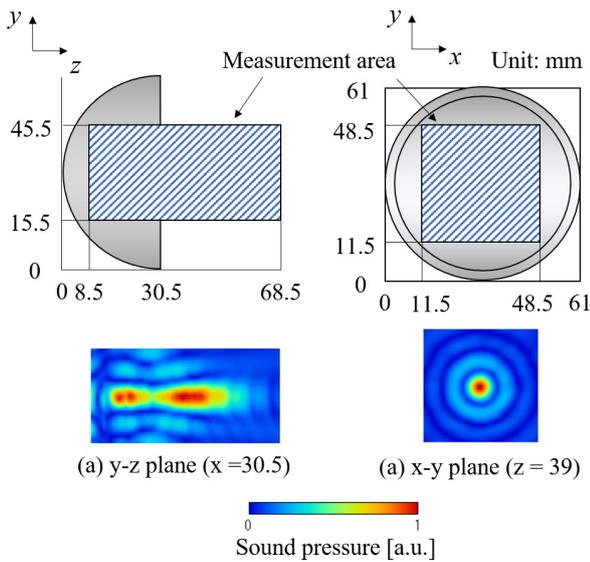
Fig. 3 Sound pressure distributions at 27.5 kHz in (a)  $y$ - $z$  plane at  $x = 30.5$  mm and (b)  $x$ - $y$  plane at  $z = 39$  mm.
