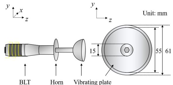
Fig. 1 Ultrasound transducer with a hemispherical vibrating plate.
