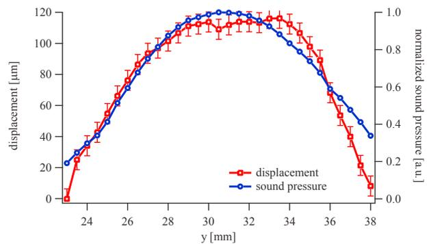
Fig. 4 Surface profile of the tissue phantom deformed by acoustic radiation force and the sound pressure amplitude distribution on the surface
