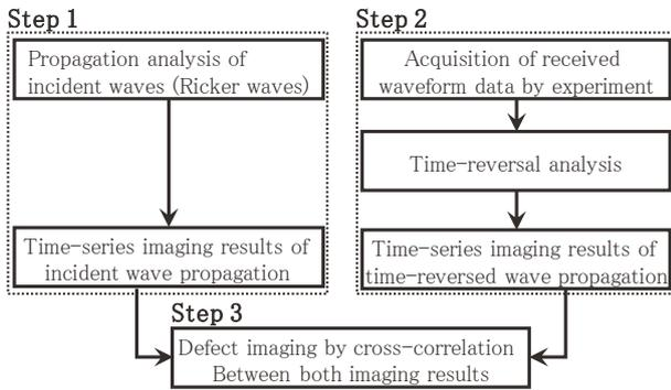
Fig. 1 Flowchart of time reversal analysis and RTM method.
