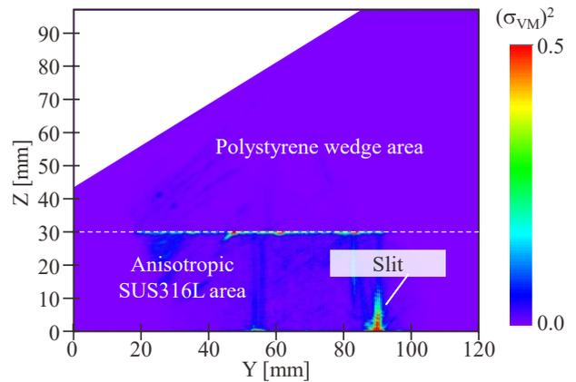
Fig. 5 Defect imaging results
