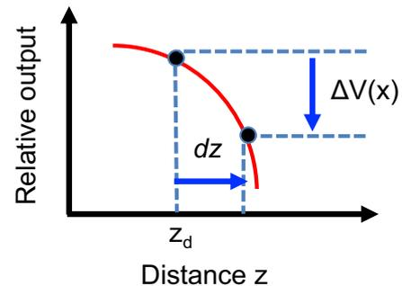
Fig. 2 Concept of  $V(x)$  method. Solid line: a part of a  $V(z)$  curve.  $z_d$ : defocus position when scanning  $V(x)$  measurement.
