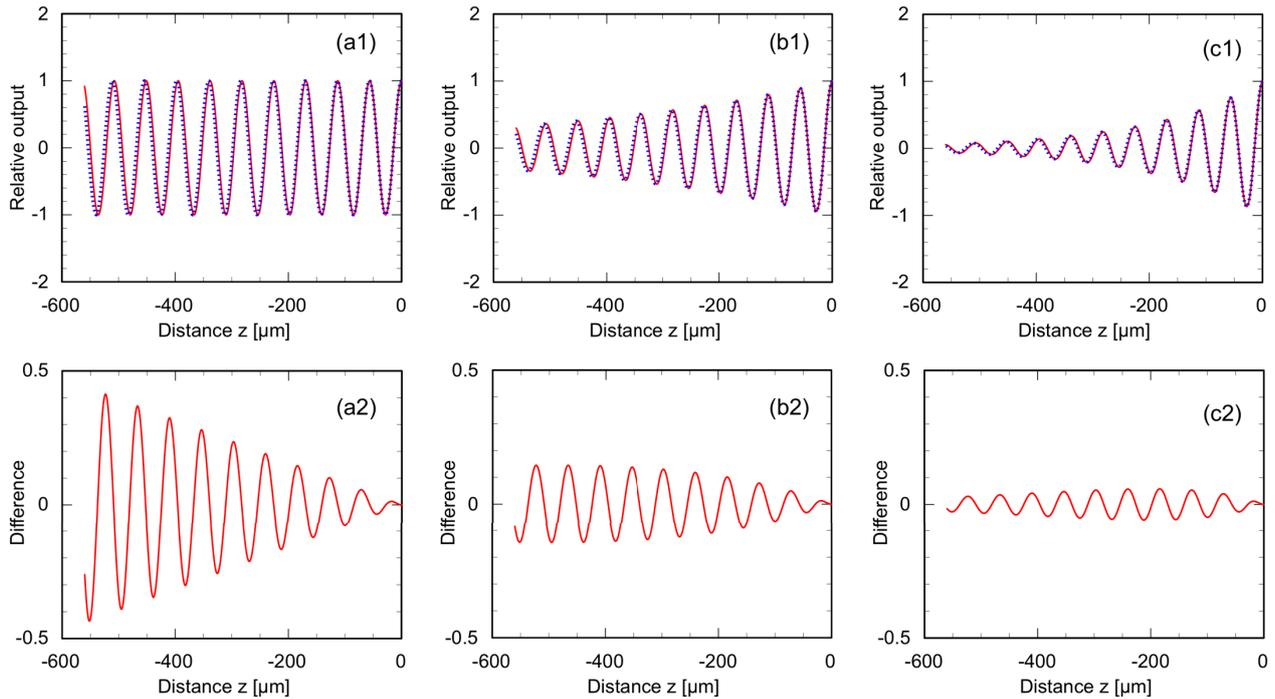
Fig. 3 Interference component of  $V(z)$  curves with different wave attenuation (upper). Interval of the waveform corresponds to LSAW velocities of 3000 m/s for solid line and 3010 m/s for dotted line at 100 MHz. Lower figures are difference between the solid line and dotted line in the upper figures. Wave attenuation  $\alpha$ : (a1)  $\alpha=0$ , (b1)  $\alpha=1/500$ , (c1)  $\alpha=1/200$  naper/ $\mu\text{m}$ .
