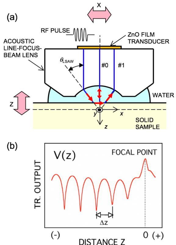
Fig. 1 Cross-sectional geometry of the LFB ultrasonic device describing the measurement principle (a), typical  $V(z)$  curve obtained as transducer output (b).
