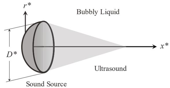
Fig. 1 Schematic of the model.
