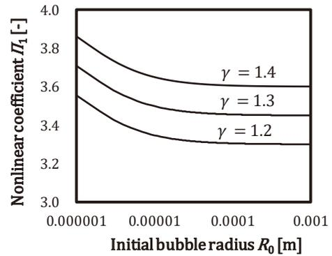
Fig. 2 Nonlinear coefficient  $\Pi_1$  versus  $R_0$  for  $\gamma = 1.4, 1.3$ , and  $1.2$  for  $\alpha_0 = 0.05$ ,  $\sqrt{\epsilon} = 0.15$ , and a normal condition of air-water system.
