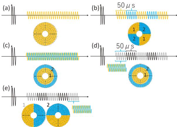
Fig.2. Schematic of ultrasonic waveform and full and split aperture.
