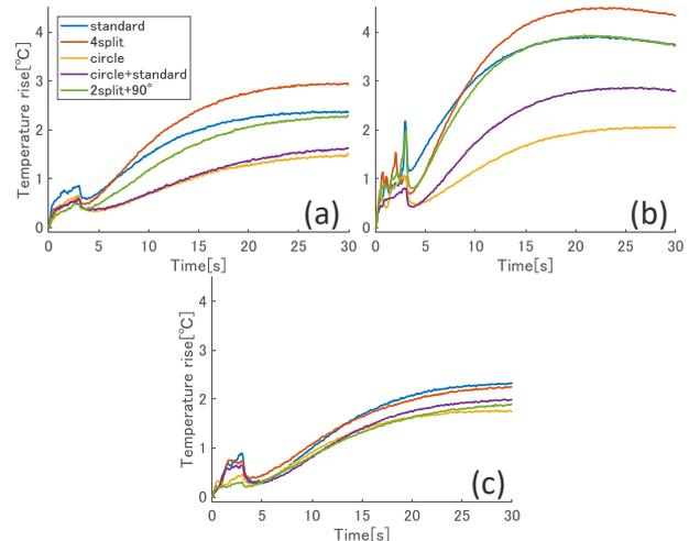
Fig.4. Temperature rise induced by sequences with five different exposure methods ( $n=3$ ) measured with thermocouples (a) in front, (b) at the center and (c) beyond.
