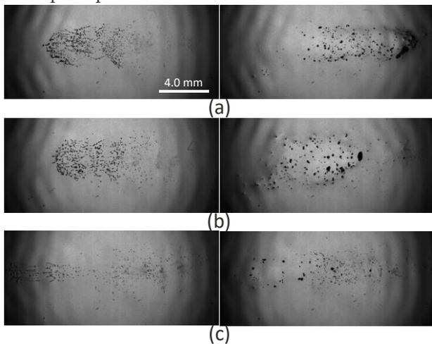
Fig.3. Images of cavitation bubbles taken by high-speed camera at 44 ms (left) and 2.99 s (right). The exposure methods were (a) standard, (b) 4 split apertures and (c) circular split focus.
