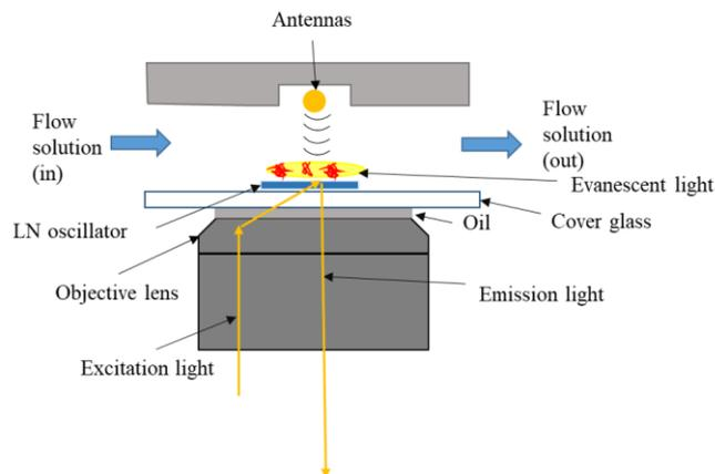
Figure 1 Schematic illustration of the experimental system.
