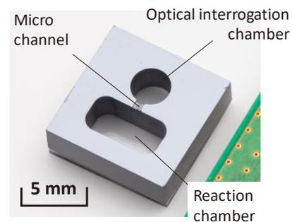
Fig. 1 Micromachined Rb gas cell
