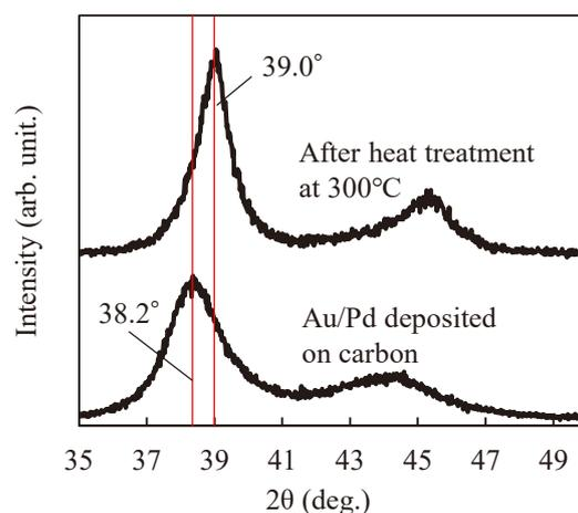
Fig. 5 XRD patterns of Au/Pd deposited carbon, before and after heating at 300°C for 1h in Ar.
