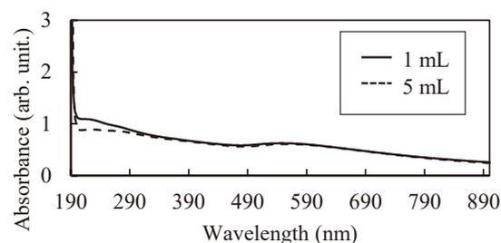
Fig. 4 UV-vis absorption spectra of Au(III)-Pd(II) solutions after ultrasound irradiation for 20 min with different amount of 2-propanol (1, 5 mL).
