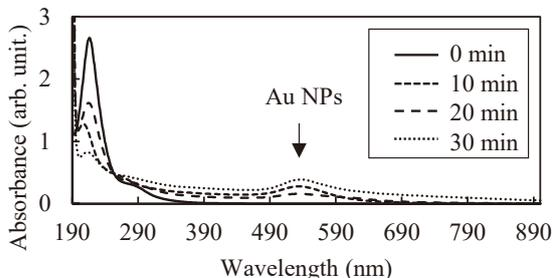
Fig. 2 UV-vis absorption spectra of Au(III) solutions after ultrasound irradiation for 0, 10, 20 and 30 min.
