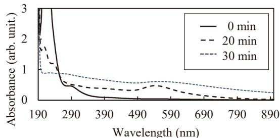
Fig. 3 UV-vis absorption spectra of Au(III)-Pd(II) solutions after ultrasound irradiation for 0, 20 and 30 min.
