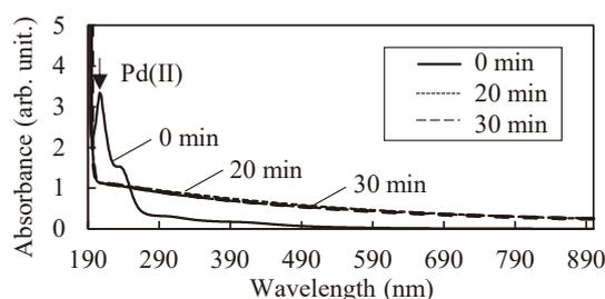
Fig. 1 UV-vis absorption spectra of Pd(II) after ultrasound irradiation for 0, 20 and 30 min.
