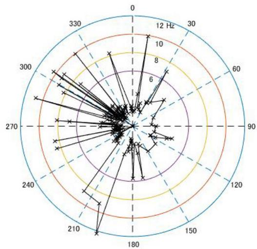
Fig.2 Principal frequency distribution with respect to azimuth for the same earthquake as in Fig.1.
