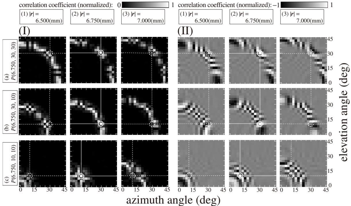
Fig. 2 Calculation results of cross-correlation coefficients using single rectangular sound source at three reflection points: (I) with squared processing for search results; (II) without squared processing for search results.
