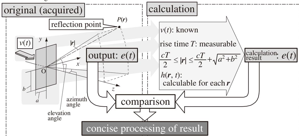
Fig. 1 Configuration of a sound source with a rectangular element and a reflection point  $P$ , and the procedure diagram for searching reflection points and obtaining search results.
