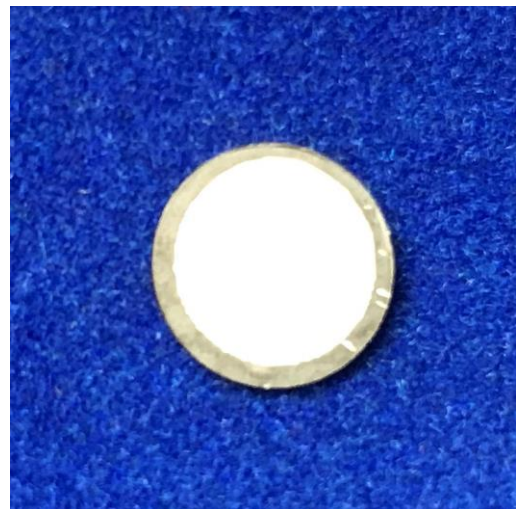
Fig. 1 The BNBTM transducer.( the diameter is 8.4mm, the thickness is 0.5mm, the electrode area is 38.5mm 2 )
