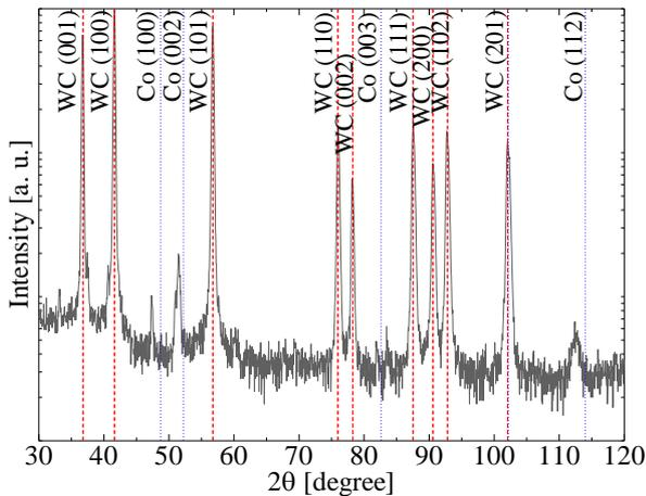
Fig. 2 XRD spectrum of WC-Co. Red and blue lines are calculated peak of WC and Co, respectively.
