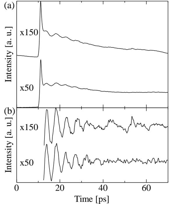
Fig. 3 (a) Reflectivity changes of WC-Co by 50- and 150-magnification objective lens and (b) extracted Brillouin oscillation.
