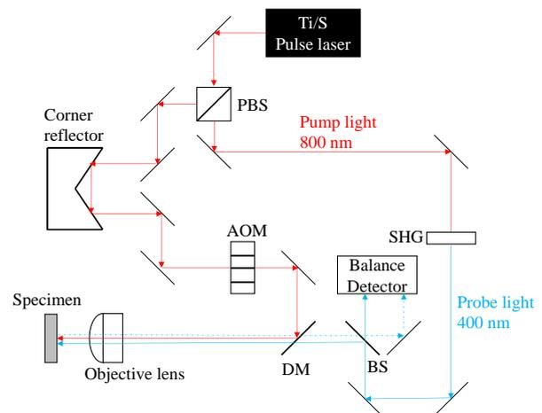
Fig. 1 Schematic of optical systems. Red and Blue lines denote pump and probe lights, respectively.
