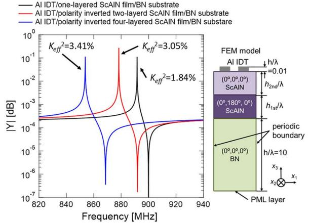
Fig. 3 The 3rd mode RSAW frequency characteristics of the admittance in Al IDT/one-layered ScAlN film/BN substrate structure, IDT/polarity inverted two-layered ScAlN films/BN substrate structure, and IDT/polarity inverted four-layered ScAlN films/BN substrate structure.
