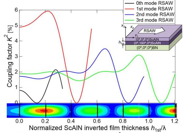
Fig. 2 The relationships between the  $K^2$  and polarity inverted ScAlN film thickness  $h_{1st}/\lambda$  on  $(0^\circ, 0^\circ, 0^\circ)$  ScAlN film/ $(0^\circ, 180^\circ, 0^\circ)$  ScAlN film/ $(0^\circ, 0^\circ, 0^\circ)$  BN substrate structure. Color map shows the particle displacement of  $x_3$  direction at resonant frequency of 3rd mode RSAW with maximum  $K^2$ .
