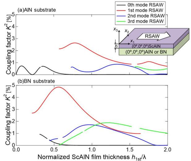
Fig. 1 The relationships between the  $K^2$  and ScAlN film thickness  $h/\lambda$  on (a)ScAlN film/AlN substrate structure and (b)ScAlN film/BN substrate structure.
