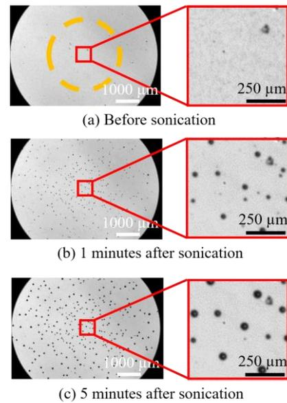
Fig. 4 Representative images of Sonazoid<sup>®</sup> microbubbles (a) before sonication, (b) 1 minute after sonication, and (c) 5 minutes after sonication. The sound frequency is 1MHz. The yellow dashed line indicates the sonication area.
