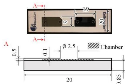
Fig. 1 Schematic of the slide-type microchamber.
