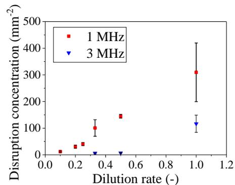
Fig. 5 Number concentration of the disrupted microbubbles. The horizontal axis was normalized by the concentration of undiluted suspension.
