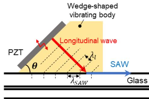
Fig. 1 Wedge transducer bonded on triple-layered glass plate.
