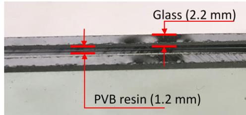
Fig. 2 Cross section of typical front shield glass.
