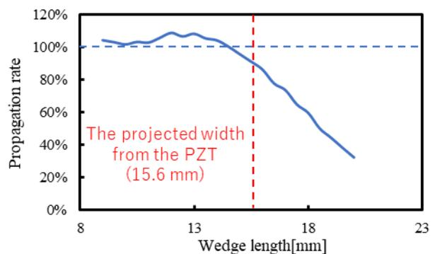
Fig.6 Propagation rate vs. bonding length.
