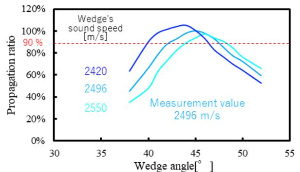
Fig.5 Propagation rate vs. wedge angle.
