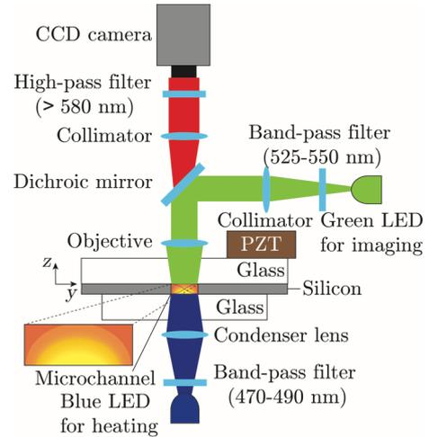
Fig. 1 Sketch of the acoustofluidic silicon chip (gray) sealed with two glass layers (white), which allows optical heating (blue LED) and particle tracking (green LED) in a volume of  $L = 1300 \mu\text{m}$ ,  $W = 760 \mu\text{m}$ , and  $H = 370 \mu\text{m}$ . The blue light is absorbed by the aqueous dye solution, which forms a temperature gradient in the channel from low (orange) to high (yellow). Reproduced with permission from Ref. [6].
