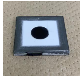
Fig.1 50µm thick BiT/TiO 2 +Sr (400°C firing) has copper and titanium top electrodes on a 5 mm thick titanium substrate
