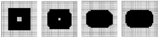
Fig.3 Topology optimization with one hole.
