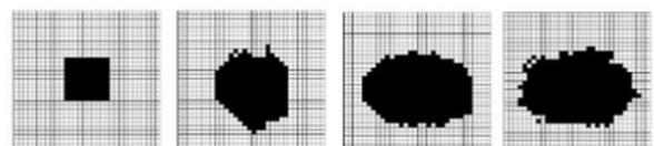
Fig.1 Structural changes during the MC step with a boundary constraint.
