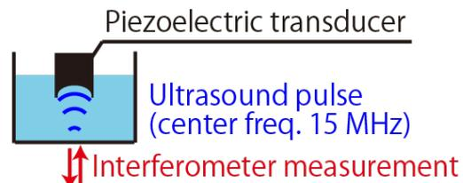
**Fig. 3** Schematic of the validation experiment. The tank filled degas water.
