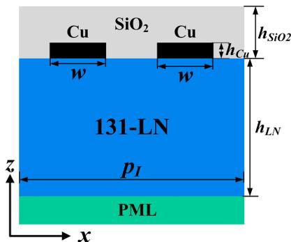
Fig. 1 sectional view of basic resonator design
