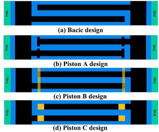
Fig. 2 Top view of four IDT patterns used for the discussion
