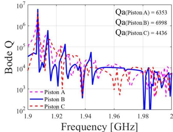
Fig. 5 Bode  $Q$  comparison of three PM designs
