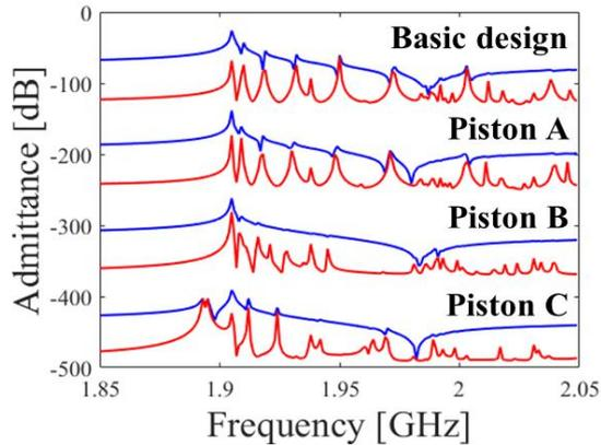
Fig. 3 Calculated admittance ( $Y$ ) and conductance ( $G$ ) of the basic TC-SAW resonator design and three Piston designs
