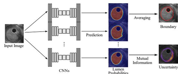
Fig. 1 Schematic of boundary and uncertainty estimation from a IVUS image using Deep Ensembles algorithm.
