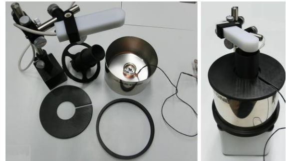
Fig. 1 Photo images of the various parts for temperature retention mechanism (left) and the assembled experimental setup (right).
