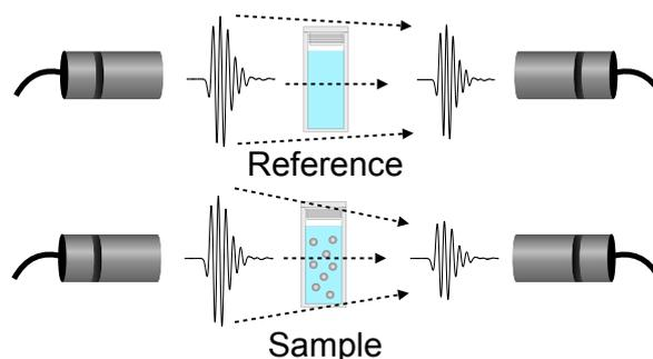
**Fig. 2** Schematic representation of the experimental setup for ultrasonic transmission spectroscopy.
