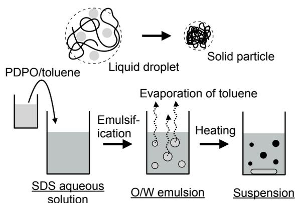
**Fig. 1** Schematic illustration of the preparation method of the PDPO particles.
