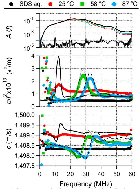
**Fig. 4** The transmission amplitude of ultrasound pulse as a function of frequency  $A(f)$  and the frequency dependences of  $\alpha/f^2$  and  $c$  of the PDPO particle suspensions. The experimental data (markers) and the theoretical calculations (lines).
