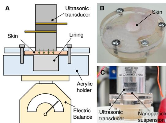
Fig. 1 Experimental setup of an ultrasonic irradiation device for sonophoresis. (A) The skin was placed on an acrylic holder, and the contacts were sensed by an electronic balance. (B) Place the skin in the acrylic holder in a taut position. (C) A suspension of nanoparticles was injected between the ultrasonic transducer and the skin for irradiation of ultrasound.
