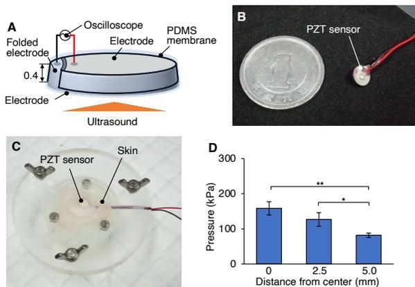
Fig. 2 Acoustic pressure measurement using PZT sensor. (A) Schematic illustration of PZT sensor and (B) a fabricated PZT sensor. (C) PZT sensor placed under the skin. (D) Acoustic pressure measured by PZT sensor.
