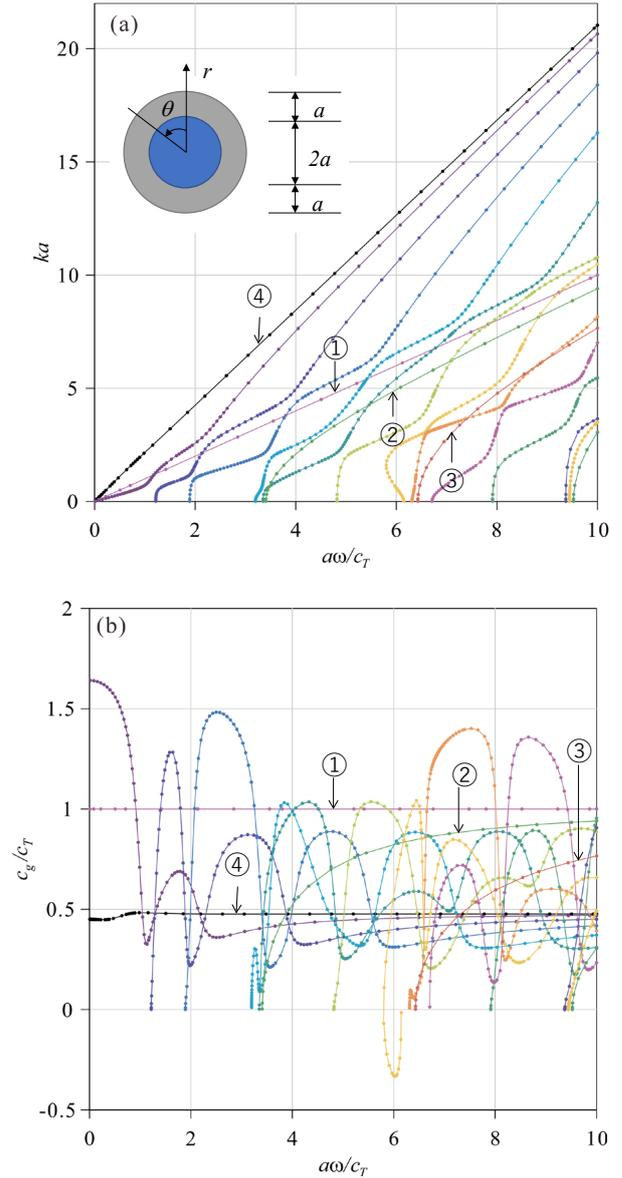
Fig. 1 (a) Frequency – wavenumber curves for an aluminum pipe filled with water. The inner and outer diameters of the pipe are  $2a$  and  $4a$ , respectively. (b) Group velocity dispersion curve.
