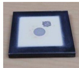
Fig.1 PT/PZT fabricated on a titanium substrate
