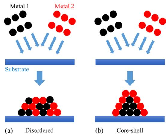
Fig. 1 Schematics of internal structure of bimetallic alloy nanoparticles. (a) Disordered structure and (b) core-shell structure.
