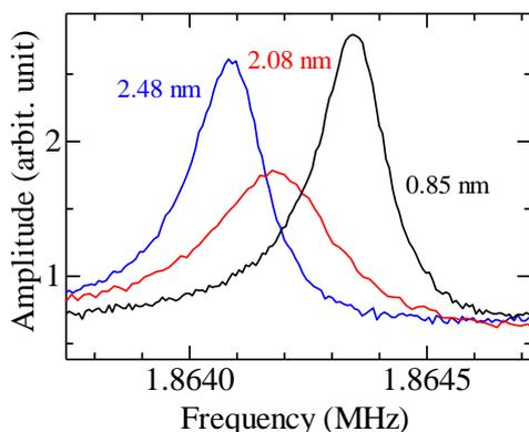
Fig. 2 Resonant spectra obtained during sputtering Pd and Au simultaneously.
