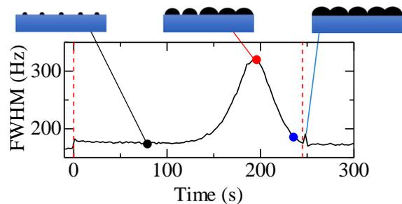
Fig. 3 FWHM during synthesizing PdAu nanoparticles. Pd and Au were sputtered during the time between dashed lines. Black, red, and blue plots correspond to the timing at which resonant spectra in Fig. 2 were obtained.
