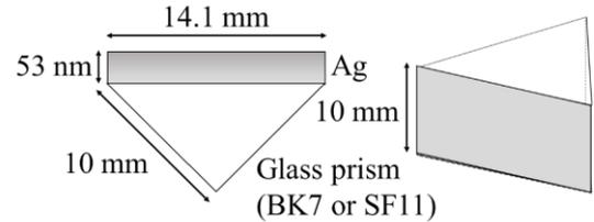
Fig. 2 Kretschmann configuration of our SPR sensors.
