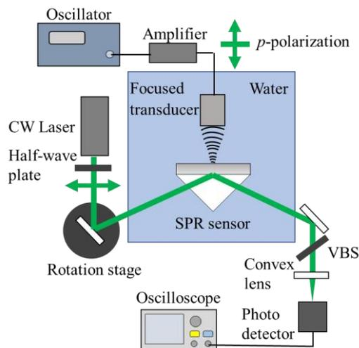
Fig. 4 Experimental system of reflectivity changes due to ultrasound radiation.
