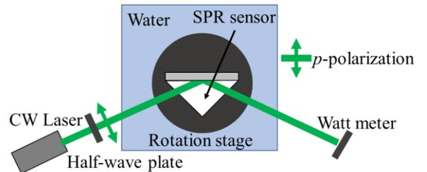
Fig. 3 Measurement system of the reflectance.
