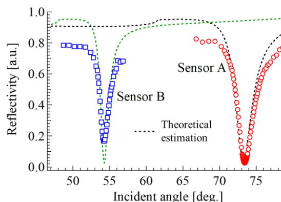
Fig. 5 Reflectance curves (experiments and theoretical estimations).
