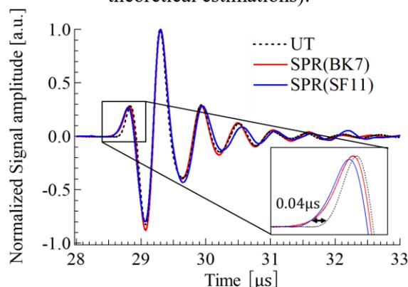
Fig. 6 Comparison of measured ultrasonic waves by SPR sensors and an ultrasonic transducer (UT).
