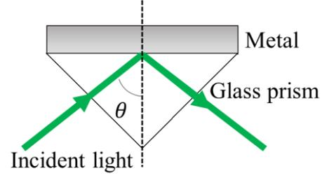
Fig. 1 A Kretschmann type SPR sensor.
