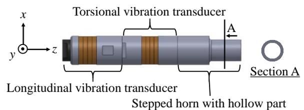
Fig. 1. Longitudinal–torsional vibration source.
