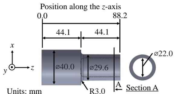
Fig. 2. Stepped horn with a hollow part.
