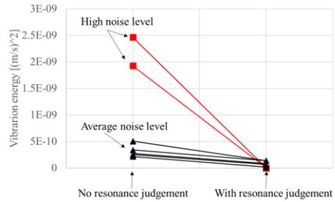
Fig.5. Difference in vibration energy before and after resonance judgement.
