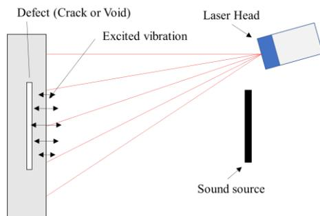
Fig.1. Schematic diagram of NCAI method.
