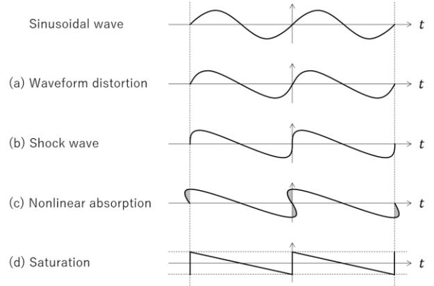
Fig. 1 Nonlinear propagation process.
