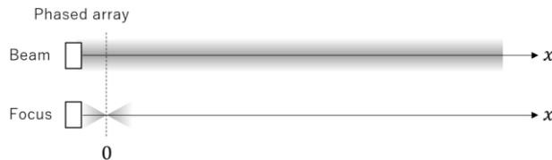
Fig. 3 Beam and focus modes of the phased array.
