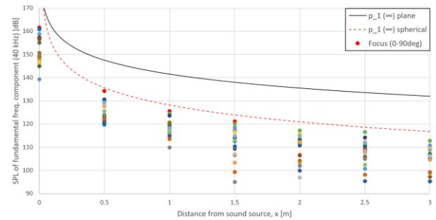
Fig. 6 Angle dependence (focus mode, maximum).
