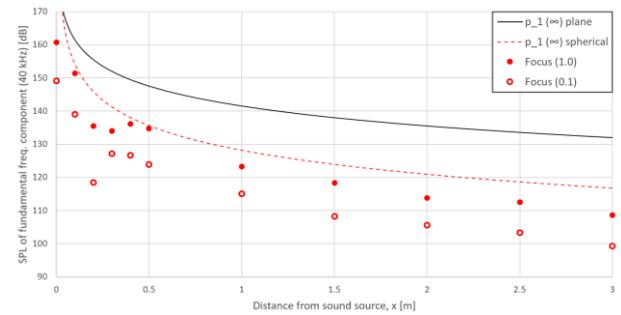
Fig. 5 Sound pressure distribution (focus mode).
