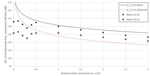
Fig. 4 Sound pressure distribution (beam mode).
