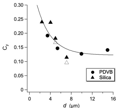
Fig. 3  $d$  dependence of  $C_y$  obtained for the PDVB and silica particles. The silica particles of  $d = 5.5$  and  $7 \mu\text{m}$  were performed in a 40 mm high polystyrene cell (open triangles). On the other hand, a polyphenylenesulfide cell with a height of 80 mm was also used to verify the effect of height (solid triangles).
