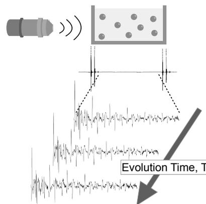
Fig. 1 Schematic representation of the dynamic ultrasound scattering (DSS) method.
