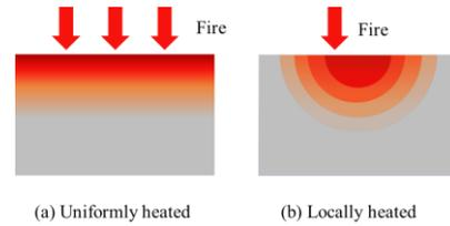
Fig. 1. Wall fire-damage model.
