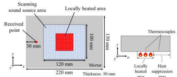
Fig. 3. Experimental sample.
