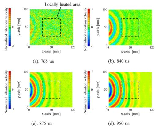
Fig. 4. Elastic surface-wave propagation results (second harmonic).
