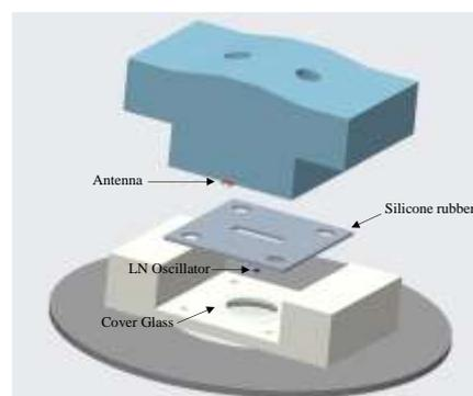
Fig. 1 Appearance of originally developed TIRFM flow-cell system with an LN oscillator.
