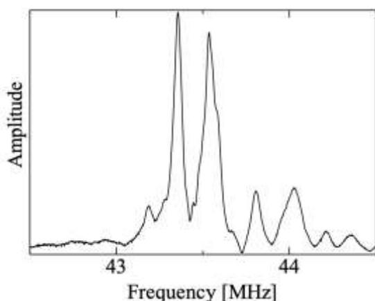
Fig. 2 Resonant spectrum of the LN oscillator during the solution flow measured by the non-contacting antennas.
