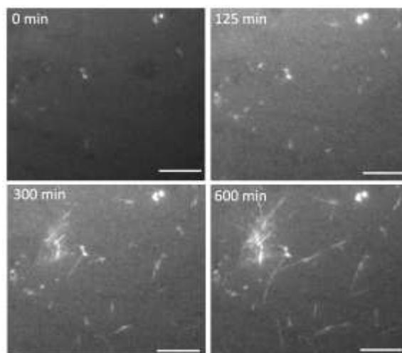
Fig. 3 Snapshots of TIRFM images on the LN oscillator during fibril elongation reaction of  $\alpha$ -synuclein. Scale bars indicate 5  $\mu$ m.
