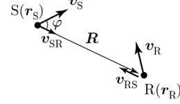
Fig.1 Positional relationship between moving sound source S and moving receiver R.
