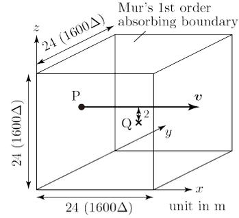
Fig.5 Numerical model for a linearly passing source or receiver.
