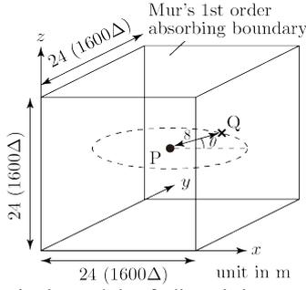
Fig.2 Numerical model of directivity analysis for fixed source or receiver.
