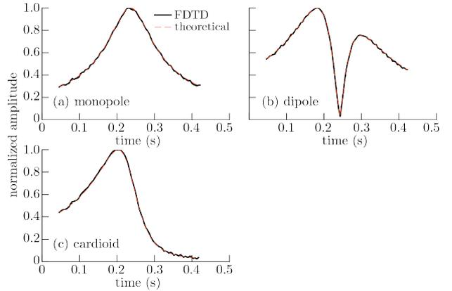
Fig.6 Normalized amplitude of a linearly passing source ( $M=0.1$ ).
