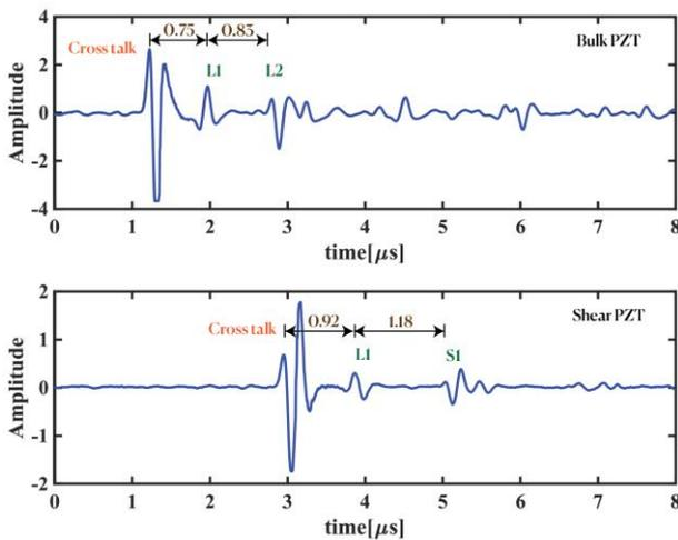
Fig. 2: Transient signal amplitude recorded at the center of the scanning area with a steel sphere, acting as a receiving electrode positioned on the opposite side of the bulk and shear PZT ceramic sample.
