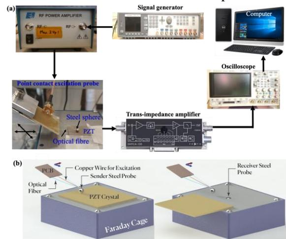
Fig. 1 (a & b) Experimental setup for point contact excitation and detection scheme for visualization of ultrasonic waves in piezo ceramics.
