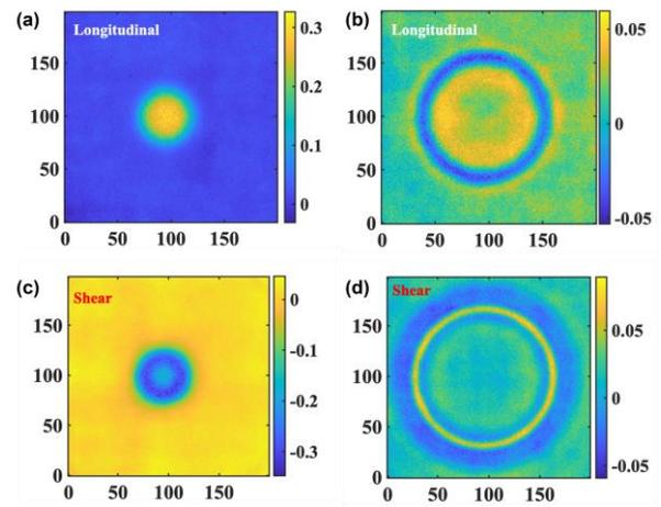
Fig. 3: Time sequential images of acoustic waves evolving in a 3 mm thick sintered bulk and shear PZT ceramic plate, (a, b) represents the longitudinal mode in bulk PZT and (c, d) represents the shear mode in shear PZT.
