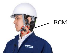
Fig. 1 An example of the bone-conduction microphone (Panasonic Corp. [1]). The microphone is placed close to the larynx.
