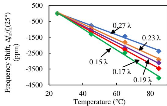
Fig. 5 Normalized anti-resonance frequency shift of SH<sub>1</sub> mode resonator as a function of temperature.
