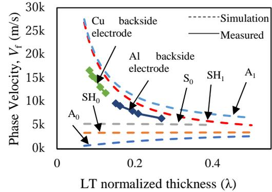
Fig. 1 Phase velocity ( $V_f$ ) of various modes of plate waves on (0°, 63°, 0°) LT with electrically shorted bottom plane as a function of LT normalized thickness.
