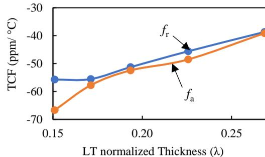
Fig. 6 Measured TCF of SH<sub>1</sub> mode resonator as a function of LT normalized thickness.
