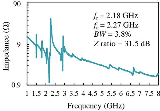
Fig. 3 Measured frequency characteristic of fabricated SH<sub>1</sub> mode plate wave resonator.
