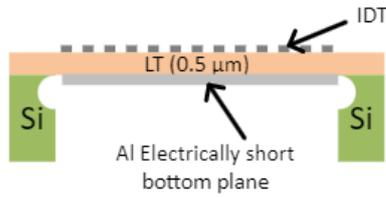
Fig. 2 Structure of fabricated SH<sub>1</sub> mode resonator.
