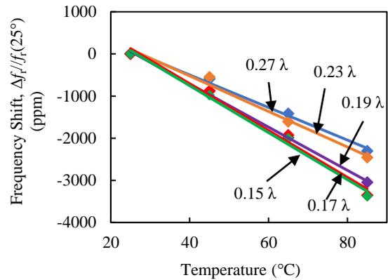
Fig. 4 Normalized resonance frequency shift of SH<sub>1</sub> mode resonator as a function of temperature.
