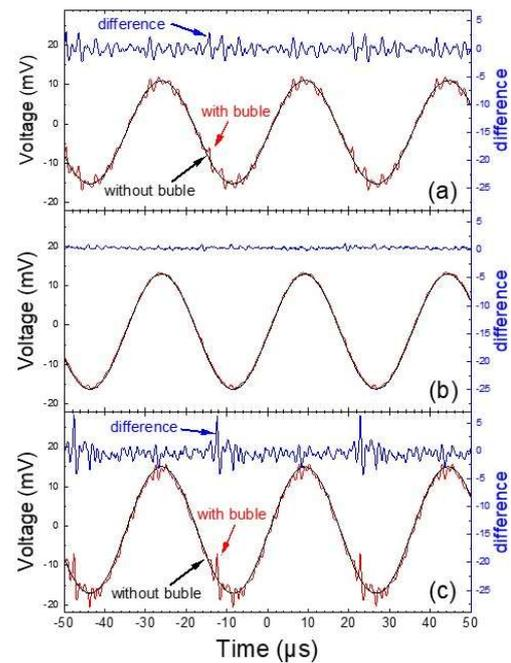
Fig. 3 AE signals from a dancing bubble (a), a stable bubble (b) and SBSL bubble (c), respectively.
