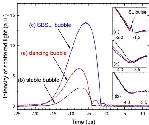
Fig. 2 Scattered-light signals from a dancing bubble (a), a stable bubble (b), and SBSL bubble (c) for one acoustic cycle. Inset: scattered-light signals enlarged in the time region where bubble contracts.
