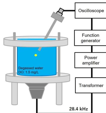
Fig. 1 Schematic diagram of the experimental system of AE measurement.
