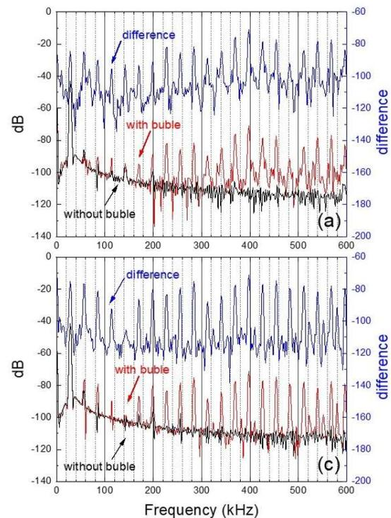
Fig. 4 Power spectra calculated from AE signals of (a) a dancing bubble and (c) SBSL bubble in Fig.3.
