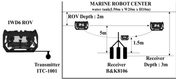
Fig. 2 The experimental configuration.
