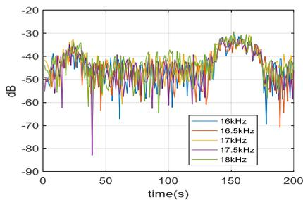
Fig. 4 Change of mark frequency energy of channel according to ROV movement.
