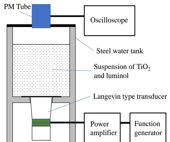
Fig. 1 Experimental setup for evaluating the amount of superoxide anion radical.
