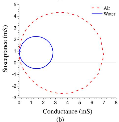
Fig. 2 Input admittance of Langevin-type ultrasonic transducer. Admittance for the water as acoustic load (a) and admittance loci for air and water as acoustic load (b).
