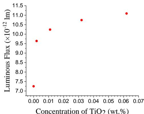
Fig. 3 The luminescence intensity change with TiO<sub>2</sub> concentration.
