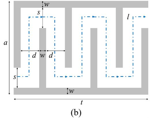
Fig. 1 (a) Underwater acoustic metamaterials<sup>5)</sup> and (b) its cross-section view of metamaterial slab.
