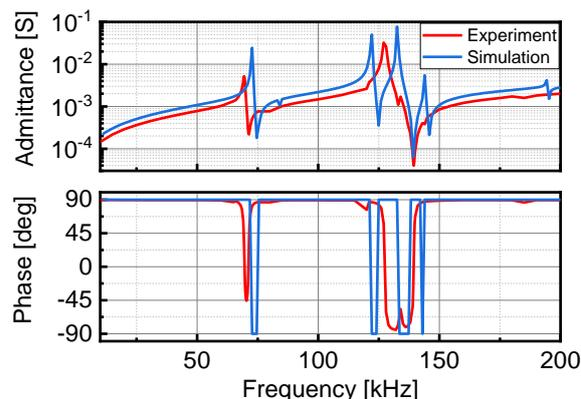
Fig. 3 Experimental (red) and simulated (blue) frequency responses of electrical admittance.
