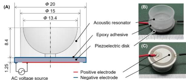
Fig. 1 (A) Profile and dimensions, and (B-C) top and bottom side views of the proposed ultrasound transducer.
