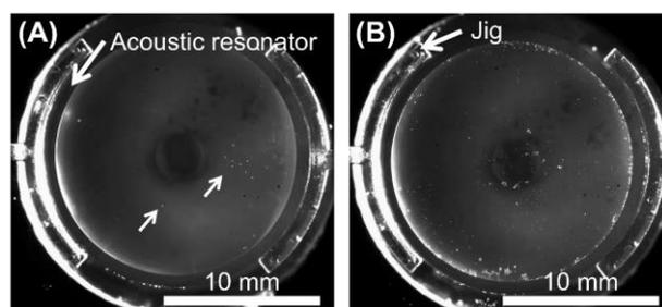
Fig. 4 Ultrasound cavitation on urethane gel under ultrasound irradiation photographed for 10 sec by high-speed camera at 250 frame/sec: Applied voltage are (A) 10 V<sub>pk</sub> and (B) 40 V<sub>pk</sub>. The operating frequency for both (A) and (B) is 127 kHz. The inside of the acoustic resonator is illuminated by a high-brightness LED. The arrows indicate the location of ultrasound cavitation yield.
