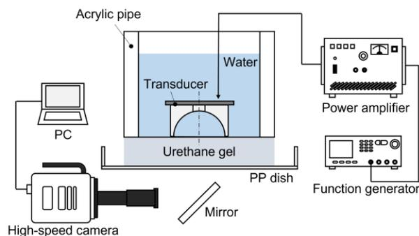
Fig. 2 Schematic of the experimental setup for high-speed imaging under sound irradiation.
