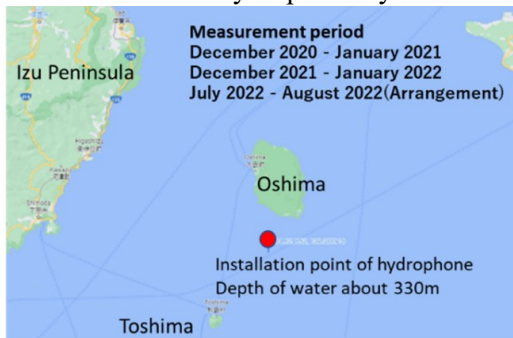
Fig. 1 Measurement Sea area and location of hydrophone system
