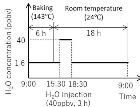
Fig. 2 Diagram of sequence of thermal desorption and TM injection.
