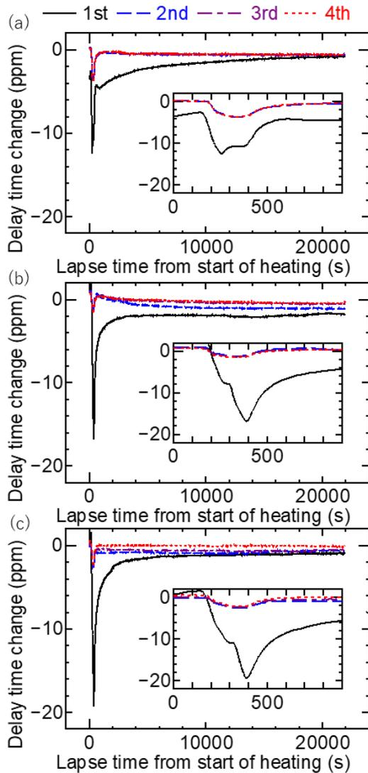
Fig. 3 Thermal desorption at 143°C with 1.6 ppbv N<sub>2</sub> flow showing samples (a) A, (b) B, and (c) C. Each inset represents the magnification of initial response.
