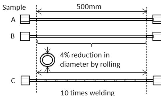
Fig. 1 Samples of the stainless-steel tubing with damaged inner surface of EP treatment. (a) raw [A], (b) radially rolled [B], and (c) welded [C] tube samples.
