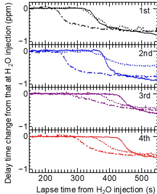
Fig. 4 Variation in TM passage by successive thermal desorption, where solid, dotted, and chained curves represent the results of samples A, B, and C, respectively.
