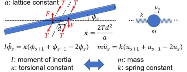
Fig. 1 The correspondence between a wave machine and a mass-spring model.
