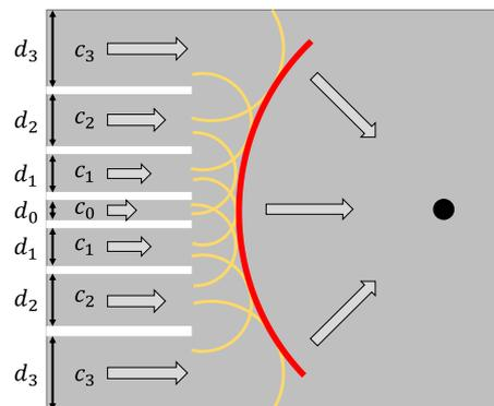
Fig.3 Schematic figure of ultrasonic focusing by designing a stacked thin plate region.
