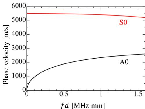
Fig. 1 Phase velocity dispersion curves of Lamb waves.
