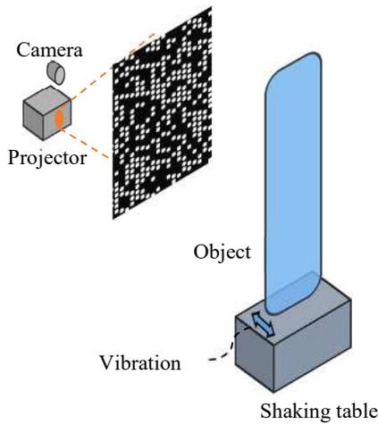
Fig. 2 A vibration measurement arrangement
