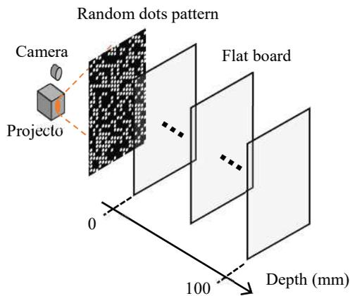
Fig.1 An arrangement for the range estimation process.
