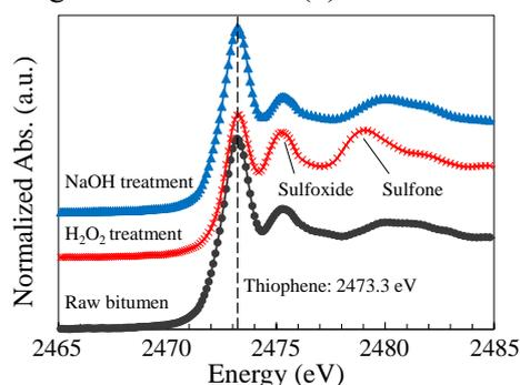
**Fig. 3** XANES spectrum of bitumen after each treatment at experimental condition A.
