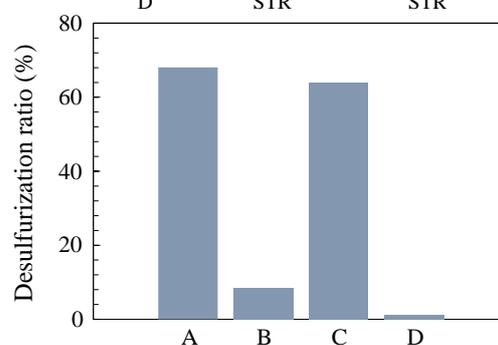
**Fig. 1** Desulfurization ratio of bitumen treated by each experimental condition.
