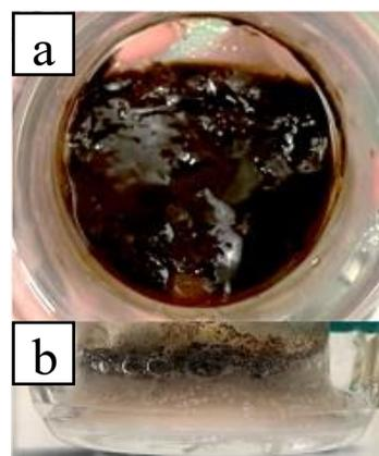
**Fig. 2** Appearance of the bitumen in solutions after H<sub>2</sub>O<sub>2</sub> treatment (a) and during NaOH treatment (b).
